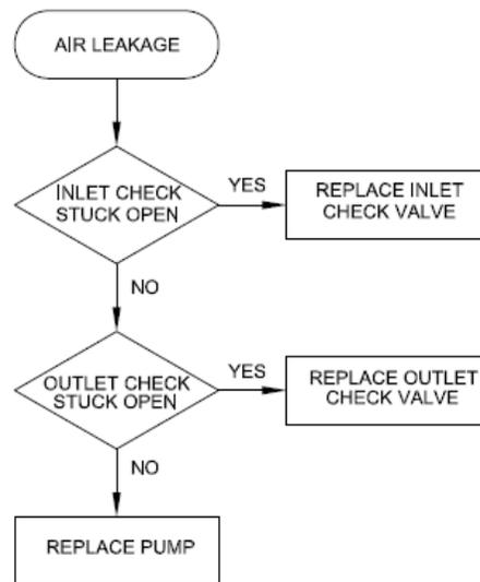
**Inlet Check Valve Stuck Open**
