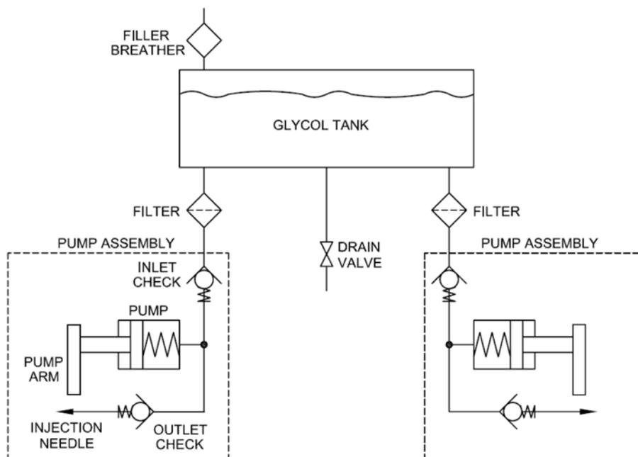
As the injection shuttle pushes a sphere towards the pump assembly, the tip of the injection needle pierces the sphere. Continued motion of the shuttle causes the sphere to press against the pump arm which compresses the piston. The inlet check valve is closed, preventing glycol from returning to the tank. As the fluid pressure in the pump cylinder rises, the outlet check valve opens, allowing the glycol in the pump cylinder to flow through the injection needle and into the sphere.
