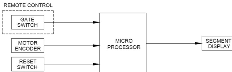
By pressing and holding the “COUNT RESET” switch, the sphere count can be reset to zero. By pressing the switch momentarily, the display can be toggled between normal display and a lifetime count of spheres indicated in thousands.
