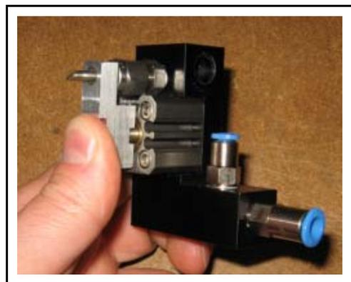
*Outlet Check Valve Stuck Shut*
