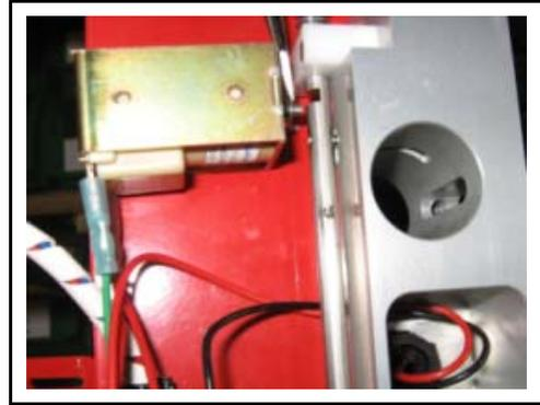
***Open Solenoid Damaged***
