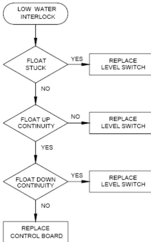
**Level Switch Damaged**
