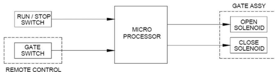
When the “RUN / STOP” switch is in the “STOP” position, the inputs from the remote control are ignored. When it is switched to the “RUN” position, there is also a short delay before the remote control signals are acted upon. This is to ensure that the hopper has time to fill its outlet queues before the gates open.
