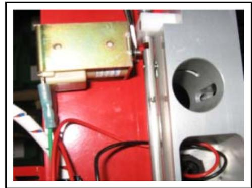
**Feed Control Rod Spring Damaged**
