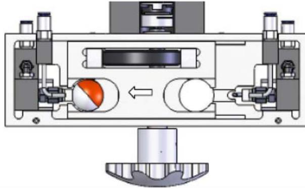
When the shuttle reverses direction, the sphere is extracted from the needle and transported to a point over the exit chute. The sphere falls through a hole in the bottom of the injection head and into the exit chute.
