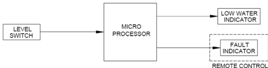
This acts as an interlock to prevent operation of the dispenser when there is insufficient water in the reservoir. A faulty connection or broken wire will also produce an open circuit, preventing operation of the dispenser.
