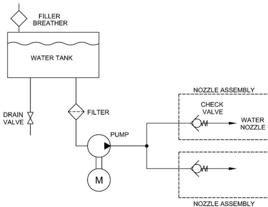
There is a filter in the water line between the tank and the pump. It has a clear outer body to allow visual inspection. The filter can be cleaned by removing and back flushing with water.
