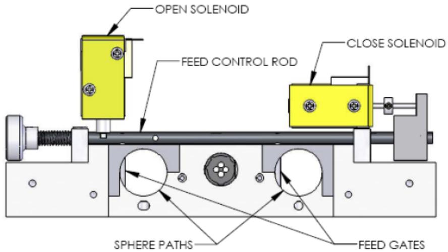
When the open solenoid is energized, it withdraws a spring loaded locking pin from the groove in the feed control rod. Once the feed control rod is unlocked, the feed rod spring forces the feed control rod to move outwards, unblocking the sphere paths.
