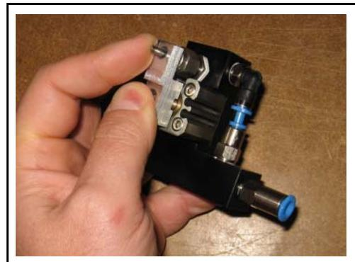
**Outlet Check Valve Stuck Open**
