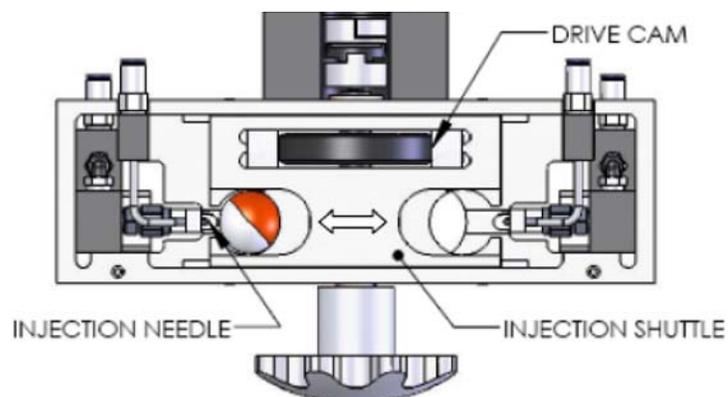
Outward motion of the shuttle causes the sphere to contact the injection needle and be injected with glycol. For details of the injection process, see *Section 3: Glycol System*.
