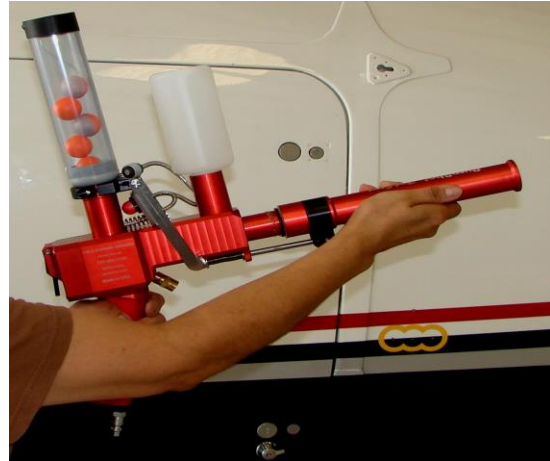
Figure 3: The injector mechanism is moved forward to the neutral position, extracting the needle from the sphere. The barrel is then moved forward in the receiver, allowing the injected sphere to drop into the receiver. (If two spheres are to be launched, a second sphere may be injected and loaded at this point. The chamber is designed for two rounds.)
